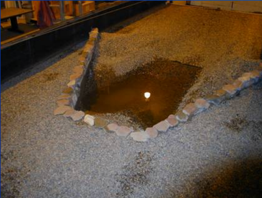
Scour hole downstream of a U-weir after testing.
